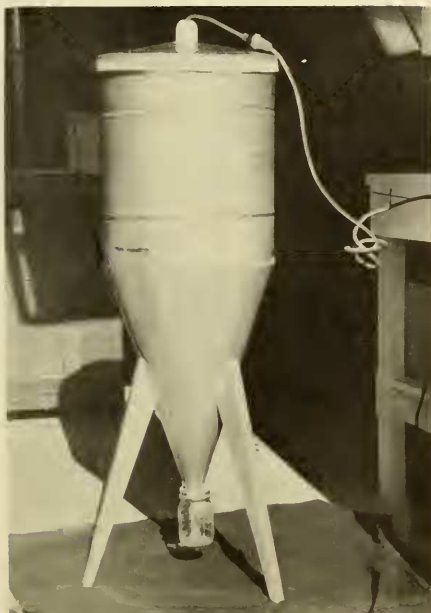
Figure 4. Berlese funnel used for extraction of arthropods.
